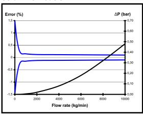
For serial (single pipe/path) sanitary design Qmax is 6000 kg/min (50%) Error of reading (including zero drift) indications refer to reference conditions  $H_2O$ ,  $18-24^{\circ}C$  (66-76°F), 1-3 bar (15-45 psi) Pressure drop refers to Newton liquids, with parallel measuring loops and sealless construction Nominal flow refers to approx. 10 m/s (33 ft/sec) velocity in measuring loops for best performance Calibration to customer range possible
